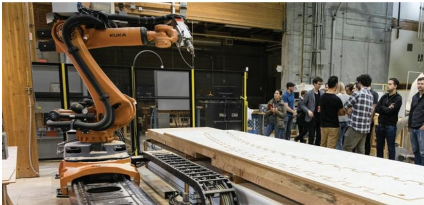
A new robot milling cell with the capability of machining wood panels up to seven metres long, working in eight axes of motion, is helping the Centre for Advanced Wood Processing (CAWP) research and develop complex free-form wood structures that previously existed only in virtual environments. The robot comes from Kuka Roboter GmbH, one of the world's largest robot manufacturers, and is the first of its kind in Canada.
