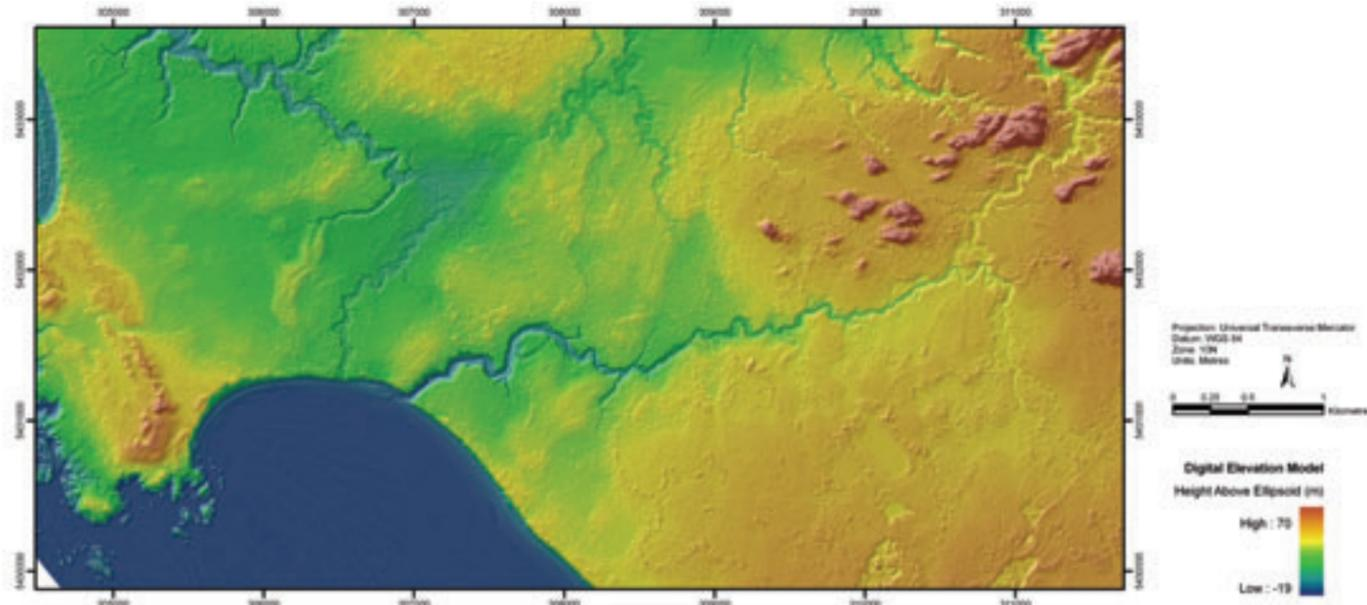
Bald Earth digital elevation model of Clayoquot Sound, derived from the LiDAR pulses which reached the ground, through the forest canopy.
