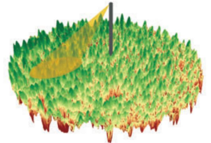
Schematic view of the Campbell River forest canopy as measured using airborne LIDAR and the view of the spectro-radiometer.
